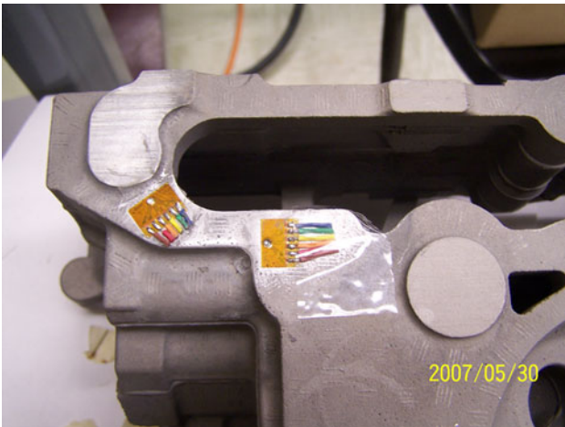
Fig. 16 Residual stress measurement locations on cylinder head
